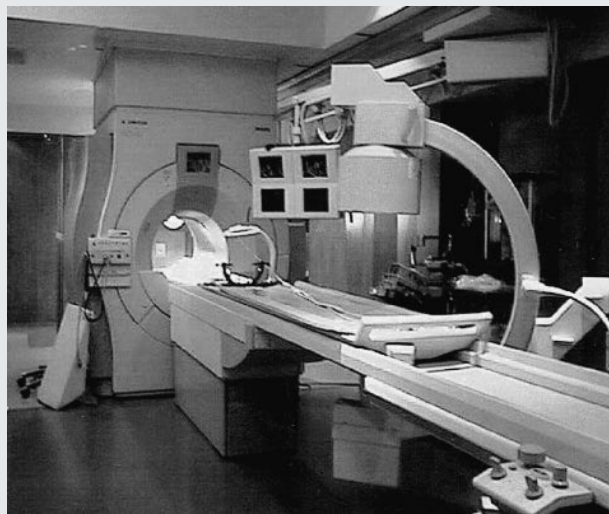
Fig 1. Superconducting short-bore system. The solution proposed by Phillips, cited in this example at the University of Minnesota, includes a standard short-bore superconducting 1.5 T MR imager adjacent to a surgical work-space that includes C-arm fluoroscopy. A custom table can slide from the surgical work-space into the magnet for intermittent imaging at appropriate times during the surgical intervention. The C-arm fluoroscopic unit can also assist with angiographic procedures. (Photo courtesy of Charles L. Truwit, MD, University of Minnesota)
