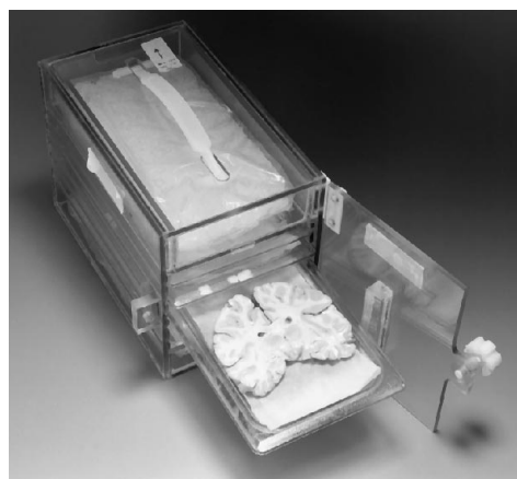
Fig 1. Brain slice holder with a brain slice on one of the five trays.
