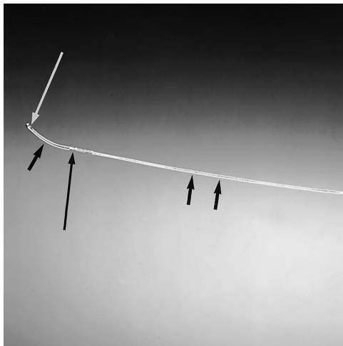
Fig 5. The distal end of the detachable endovascular electrocoagulation device shows stainless steel delivery wire ( double arrows ); uninsulated steel junction ( long black arrow ); crescent-shaped 6-mm long platinum coil ( short arrow ). The distal, 1-mm, portion of the platinum coil is insulated ( white arrow ) to avoid possible convergence of the RF energy in a too-small area of the vessel.
