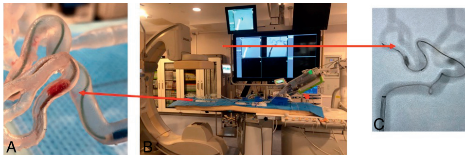
FIG 1. A benchtop 3D printed vascular model with a thrombus inside (A) was connected to a Corindus CorPath GRX robot (B, arrowhead), and MT was performed using SRs (C).
