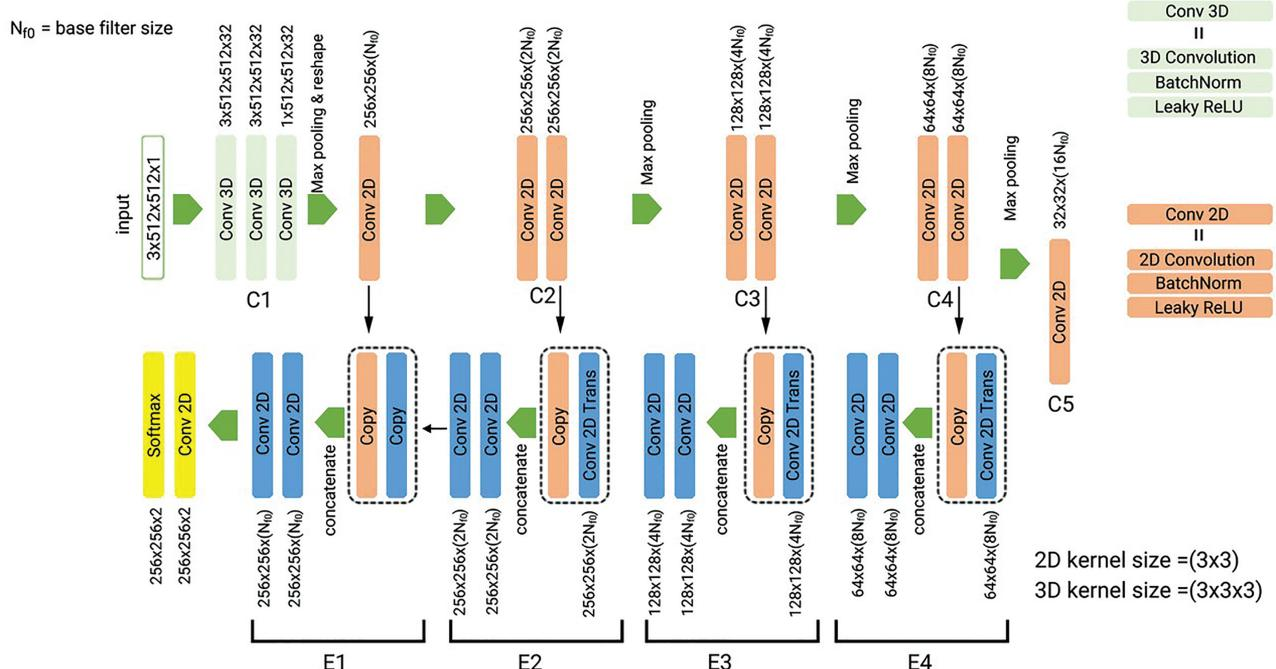
**ONLINE FIGURE.** CNN design. Schematic of the hybrid 2D–3D CNN used by RAPID for ICH detection.
