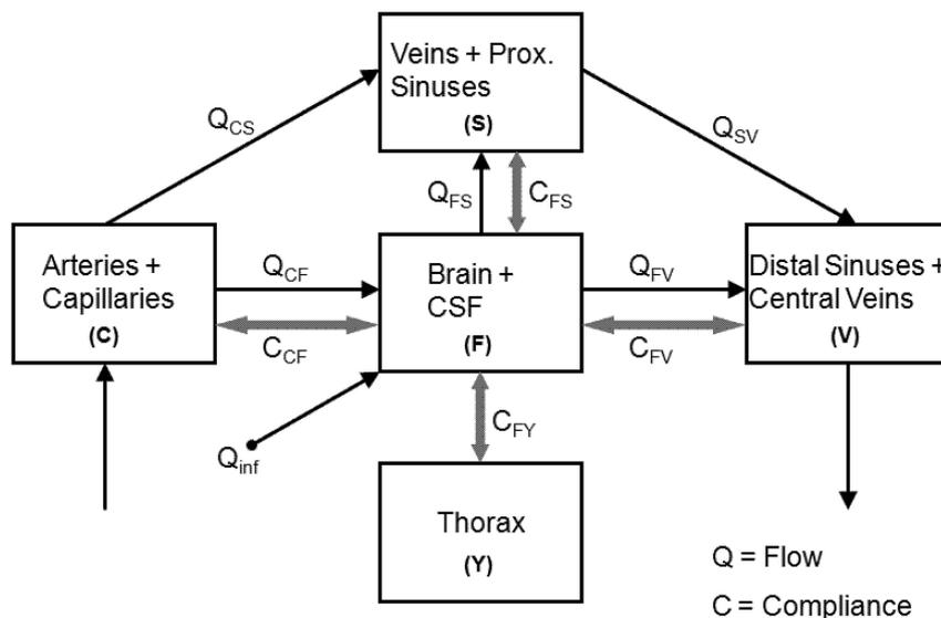
**Fig A1.** Compartmental model of intracranial pressure and volume dynamics. Flow rates between various compartments are represented by  $Q_{ij}$ , and compliance of membranes between compartments are represented by  $C_{ij}$ . The model includes a Starling-like resistor between compartments  $S$  and  $V$ , modeling a collapsible venous sinus, such that  $Q_{SV}$  also depends on CSF pressure.
