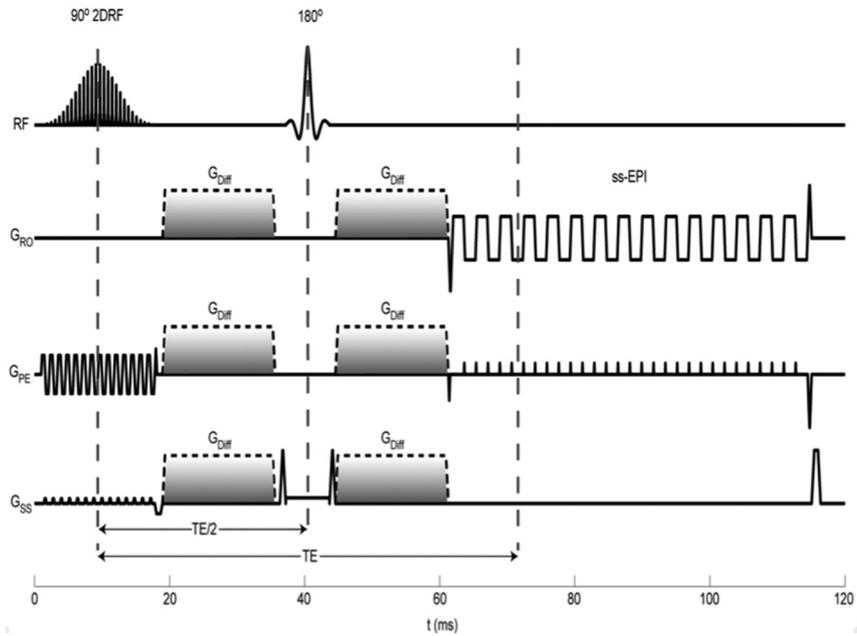
**On-line Fig 1.** Example of the pulse sequence timing diagram for the rFOV DWI sequence. Further information can be found in reference 45.
