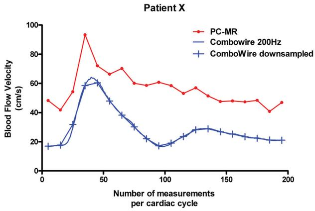
**On-line Fig 1.** Velocity data acquired by the ComboWire down-sampled to match the number of measurements obtained with PC-MR imaging compressed.
