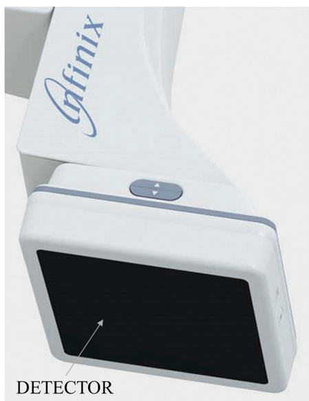
ON-LINE FIG 1. Photograph of the new x-ray imaging system. The detector has both a regular-resolution 194- \mu\text{m} pixel FPD mode and a high-resolution 76- \mu\text{m} pixel HiDef mode in 1 single unit.
