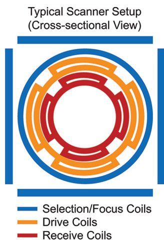
ON-LINE FIG 2. Multiple coil sets are combined to generate all required fields in the 3 anatomic axes, including selection/focus-field coils (blue), drive-field coils (orange), and receive coils (red).
