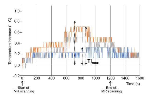
On-line Fig. 1 Chronological changes in temperature increase (TI) for ΤI three locations the right-angled clip.  $(^{\circ}C)$ at indicates the difference between temperature before magnetic resonance (MR) scanning and during or after MR scanning (latter - former). Blue, orange, and grey lines denote TI at the tip of the clip head, angled part of the clip, and 5 mm from the tip of the clip head, respectively.  $TI_{max}$  denotes maximum TI at each location.
